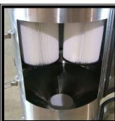
On the back of the machine - the upper door opens to allow access to the filter/intake chamber – the lower door opens to allow access to the removable five gallon dirt bucket
